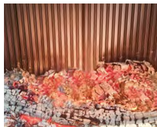
Bed of embers without flames - combustion is finished
