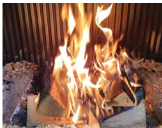
Flame pattern "Main combustion phase"
