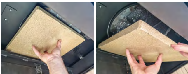
Removal of upper deflector plate
