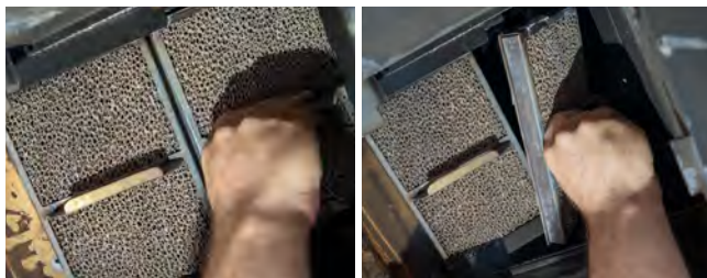
Removing the catalytic converter units for panorama formats
